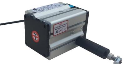
The AWP120 series are wire potentiometric position transducers that turn a linear motion into a resistance variation. They are made of a precision rotating potentiometer operated by a, winding or unwinding, stainless steel wire. The transducers are available with a stroke of: 300 to 2750 mm. Optionally other stroke lengths, cable length and socket connector can be requested.
