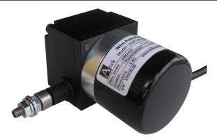
The AWP110 series are wire potentiometric position transducers that turn a linear motion into a resistance variation. They are made of a precision rotating potentiometer operated by a, winding or unwinding, stainless steel wire. The transducers are available with a stroke of: until 250 mm to 1250 mm. Optionally other stroke lengths, cable length and socket connector can be requested.
