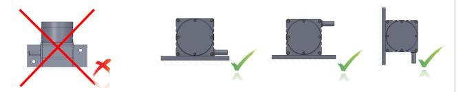
3. If there is the possibility of splashing of water (like rain) on the device, the wire outlet must not look upwards. If the wire needs to go upwards, please use guide rollers.
