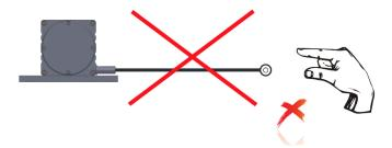
2. The wire encoder must be mounted vertically in position, not horizontally.
