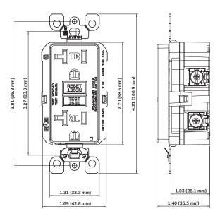
20A SmartlockPro® Self-Test GFCI
