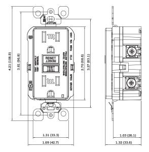
15A SmartlockPro® Self-Test GFCI
